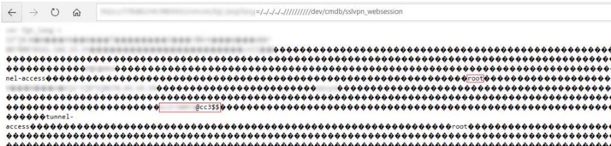
Figure 3 Directory traversal – file contains username and password in plaintext format
